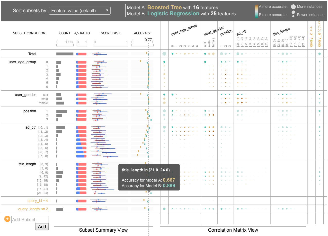
Figure 1: A screenshot of MLCube Explorer , our interactive visualization tool for analyzing and comparing machine learning results. Each row represents a subset. The subset summary view (middle) visually shows several statistics for each subset (e.g., count, proportion of positive instances, distribution of prediction scores, and model’s accuracy). The correlation matrix view (right) visualizes accuracy differences between two models for a subset combination (e.g., user_age_group=1 AND position=3 ). A cell with a larger circle means there are more instances in that subset combination. Yellow means Model A outperforming Model B; green means Model B outperforming Model A. The darker the color, the greater the performance difference. Users can interact with the interface in several ways, including drill-down, sorting subsets, and adding new subsets.
